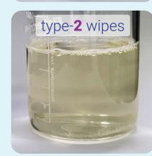
**Method:** To characterise the interaction between fibre and liquid in more detail, non-wovens were soaked in an alcoholic solution (14 g ethanol, 6 g 1-propanol, 10 g 2-propanol, ad 100 g water, pH 8) for 72 h and then the squeezed out liquid was analysed. Pictures, the pH value, and the efficacy against adenoviruses according to EN 14476 (high organic load) were determined.
