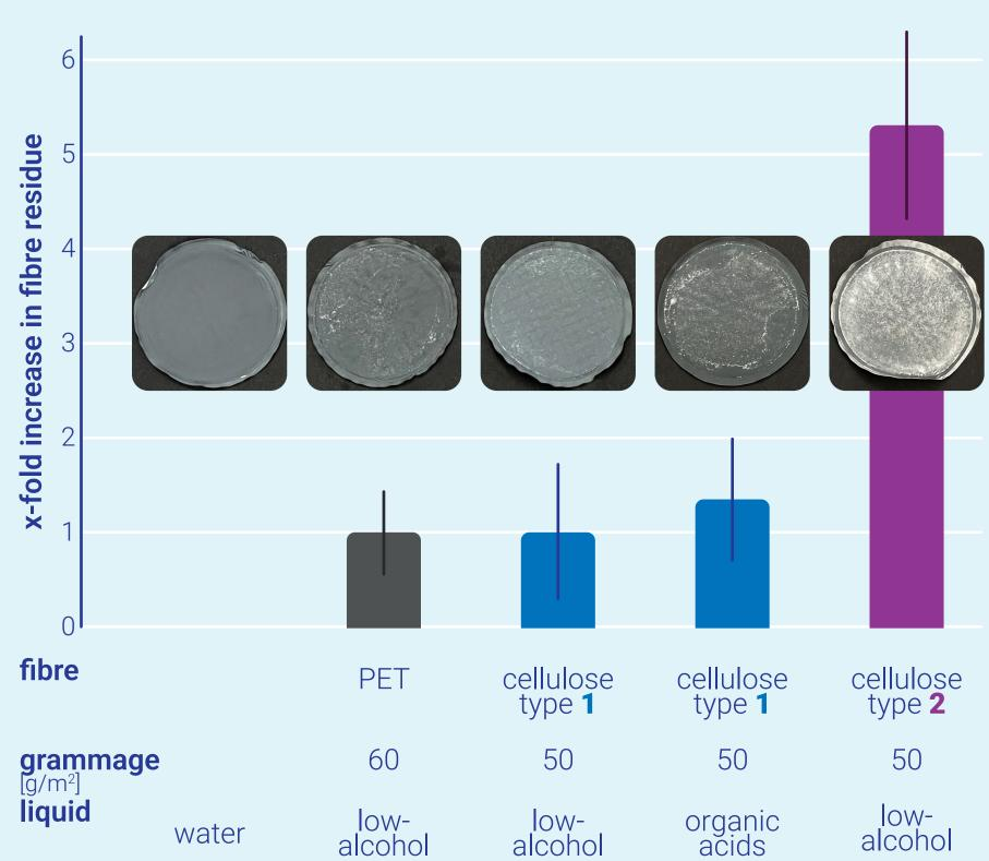
The tested pre-soaked wipes of fibre type 1 leave the same amount of lint as PET fibres. Non-woven wipes containing pulp as interlayer (type 2) leave more than five times more fibre residue.
