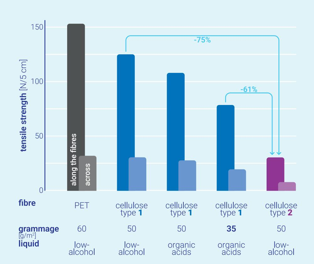
Cellulose-based non-wovens of type 1 have a slightly reduced tensile strength compared to PET fibres. However, the tensile strength of type-2 fibres is more than 75% lower than of type-1 fibres. It is even lower than that of non-wovens with lower grammage and a impregnation liquid (organic acids) that seems to reduce tensile strength in general.
