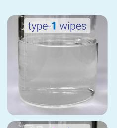
The chemical interaction of certain cellulose-based fibres with disinfectants can be seen as discolouration of the squeezed out liquid (see left pictures).
